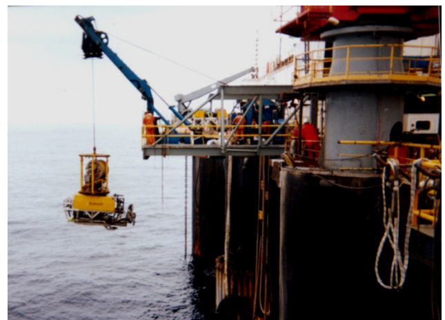
Photo showing the ROV deployment frame on the port side of the Sedco 702
