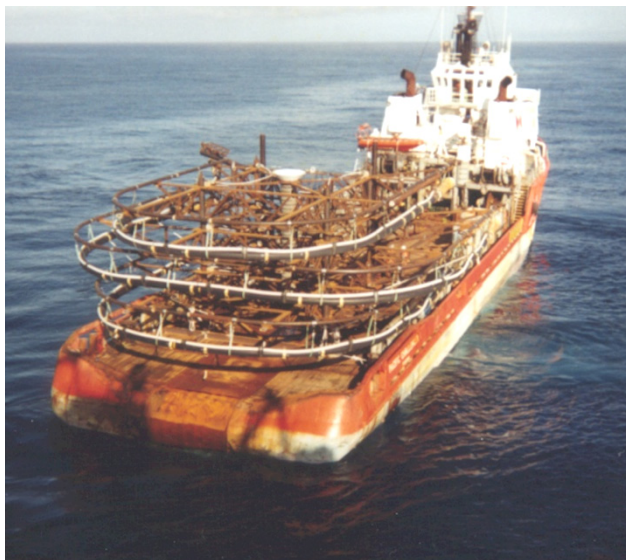
Flowline deployment frames loaded on the workboat deck
