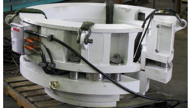
Riser Load Monitoring System – Load Ring
