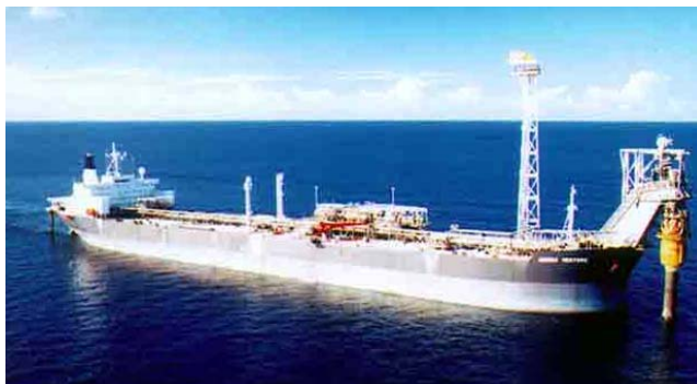
Jabiru Venture FPSO Connected to RTM
