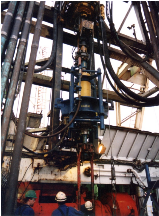
Typical Passive Heave Compensator Installation
