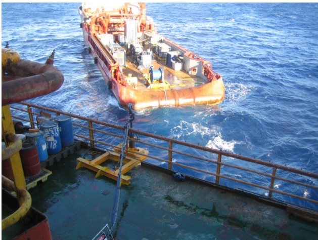
Gravel Pack Spread in Operation
