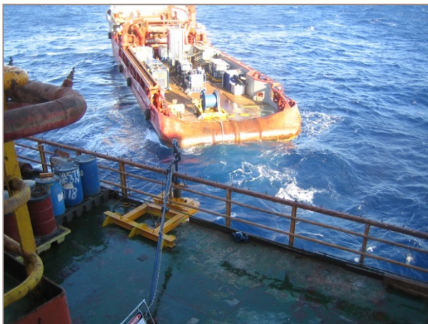
Gravel Pack Spread in Operation
