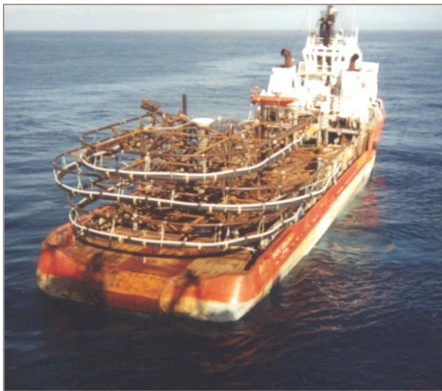
Flowline deployment Frames on the Workboat Deck
