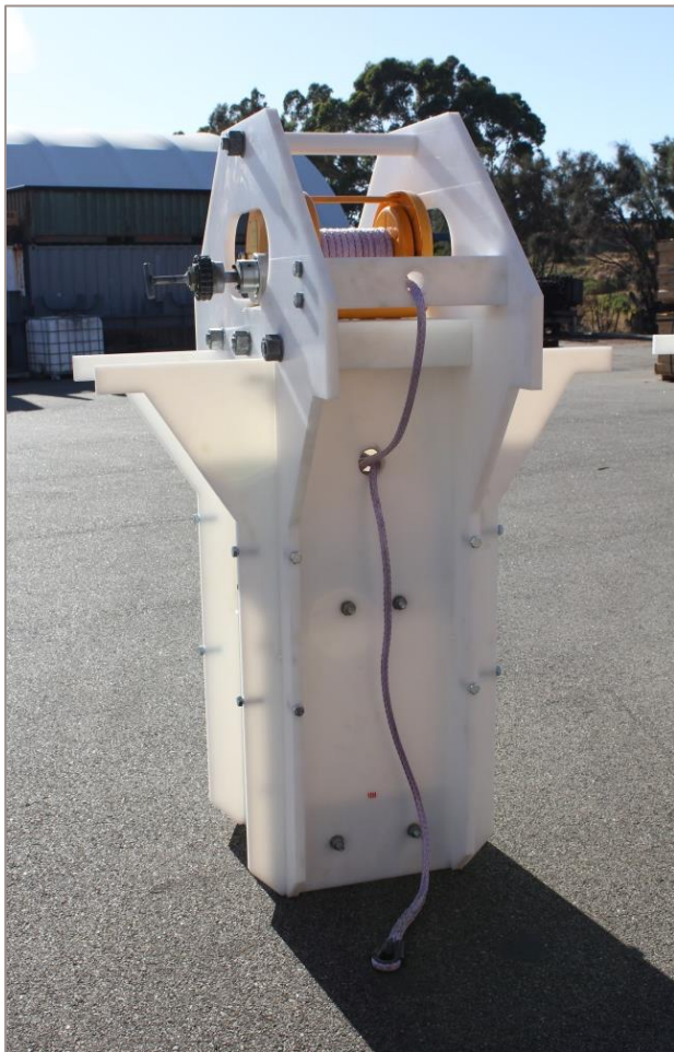
Completed taut wire unit
