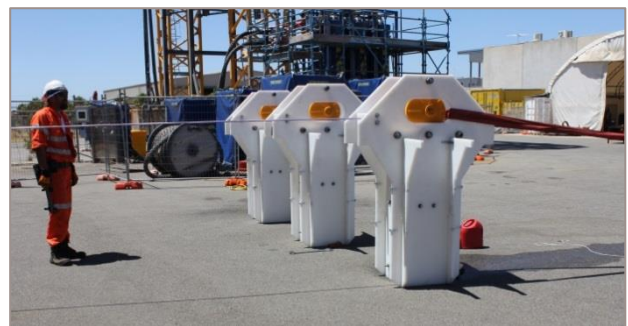
Taut wire units being tested in ICON's Henderson
