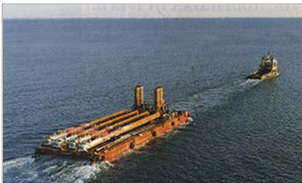
Substructures under tow to location
