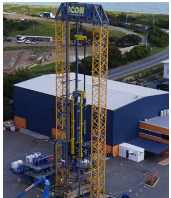
Extensive onshore testing of the ARTP E-Series proved system reliability and verified computer based design simulations with physical performance
