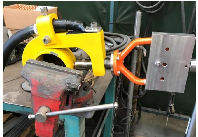
Factory Acceptance Testing a Pipe Clamp.
