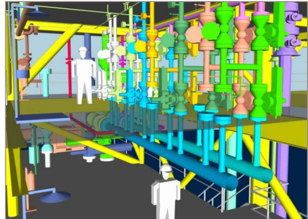
Hydraulic actuators controlled from the central processing platform will adjust well flows by activating choke valves or by diverting the product streams between manifolds. Injection of chemicals is achieved by the same method
