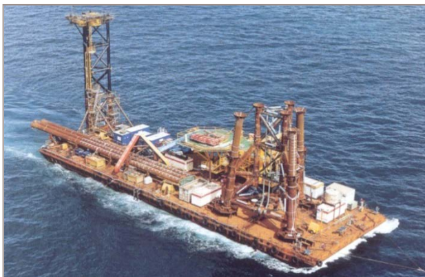
The complete structure was loaded out and transported to site on a single barge
