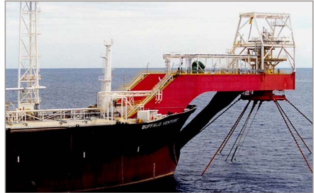
Buffalo Venture FPSO 6 Point Mooring, Riser and Control Umbilical
