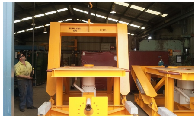
Completed PLET in Preparation for Storage
