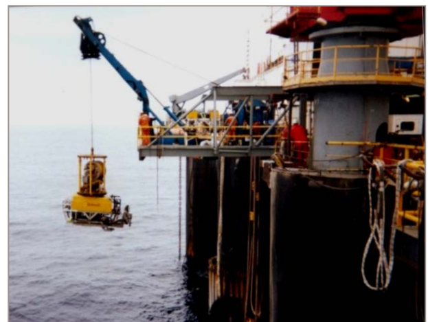
Photo showing the ROV deployment frame on the port side of the Sedco 702
