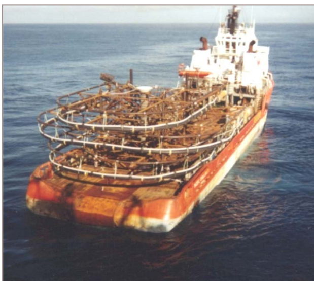
Flowline Deployment Frames on the Workboat
