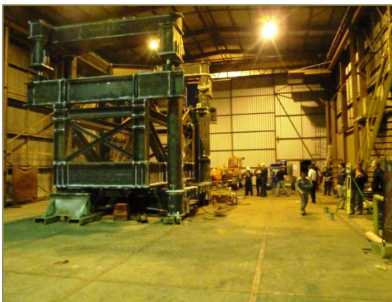
Load testing of the IFS prior to installation
