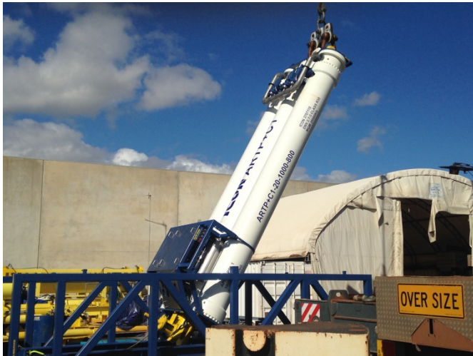
The ARTP C-Series module provides over-tension, under-tension and anti-recoil protection
